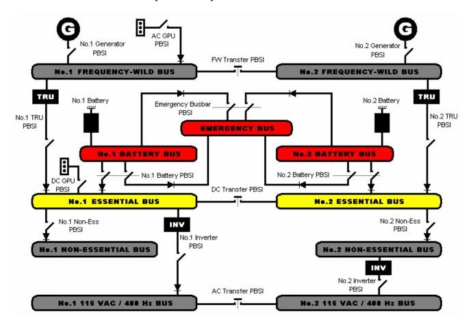
Note: on some aircraft, the n°2 inverter is powered directly from the n°2 Essential Bus. Hence it will no be shed if the Lo Volt red light comes on.
