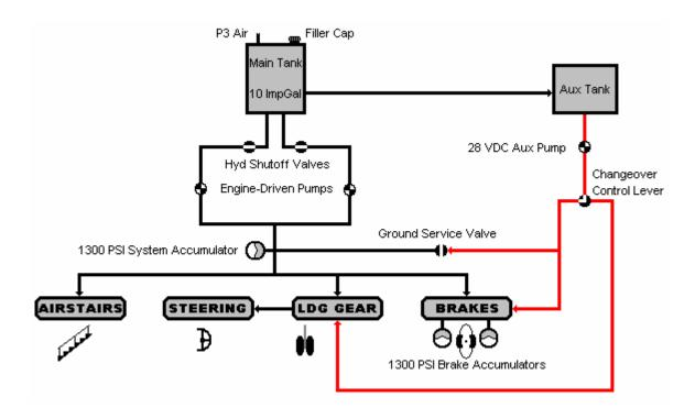
The hydraulic system is normally run by two engine-driven pumps. It allows for landing gear, power steering, brake and airstairs operation.
