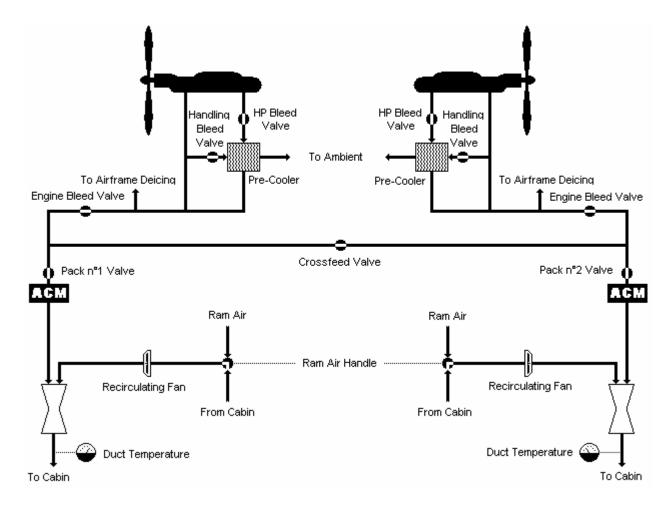
The system elects automatically whether to use only P2.5 (LP) or also P3 (HP) air in function of engine output. The HP Bleed PBSI should always be left On during normal operations, and the valve will open or close automatically. At low power settings, the HP Bleed Valve will be open, and HP air will be pre-cooled by P2,5 air coming from the Handling Bleed Valve (operated automatically to avoid compressor stall).
